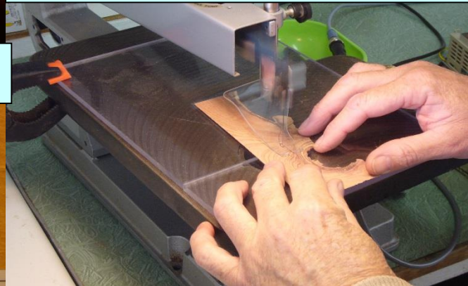
Rough shaping using scroll saw at low speed with fine blade
