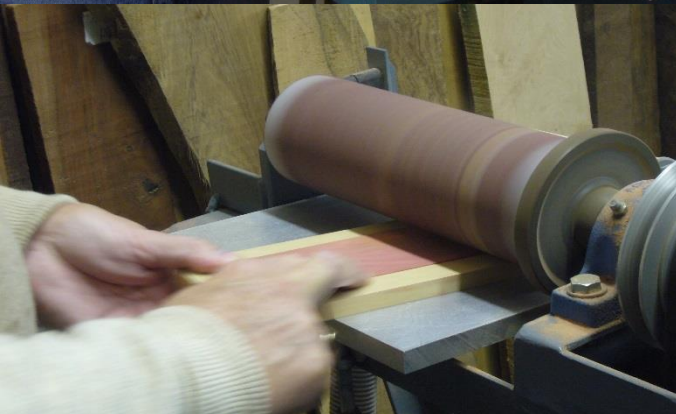
Thickening veneer with abrasive drum
