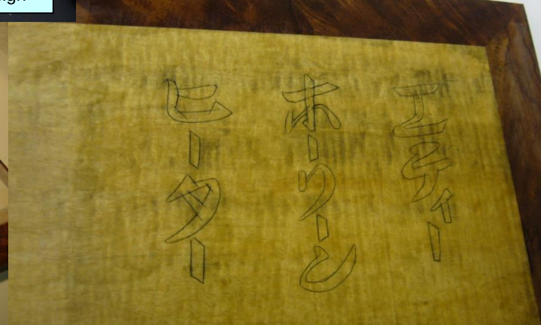
Defined edge deepened ready for routing
