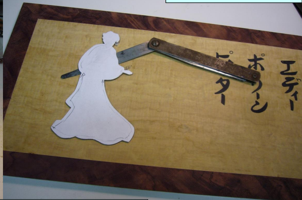
Removing from lid with feeler gauge
